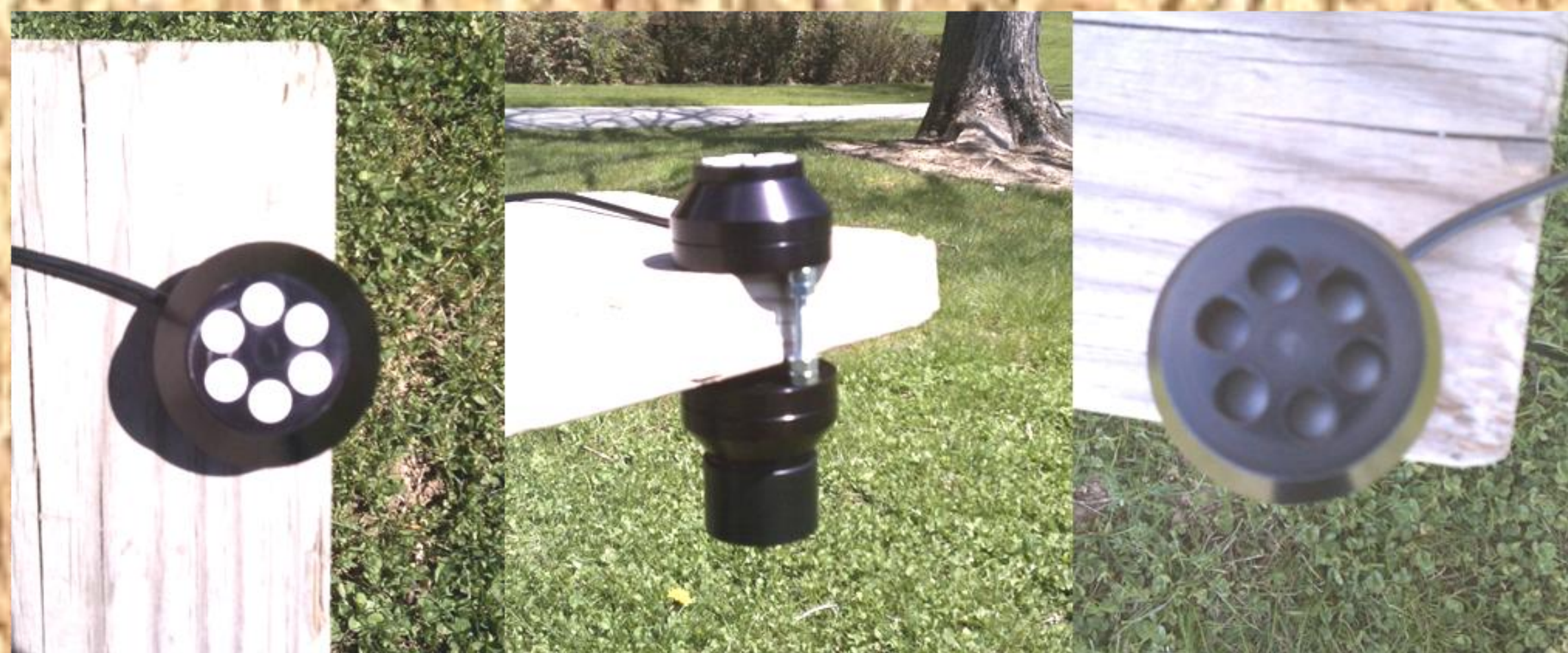
Figure 1. Triple Vegetation Index Radiometer (TVIR). From left, sensor configured to capture downwelling radiation (irradiance), combined sensor prototype, and sensor configured capture upwelling radiation (radiance).
